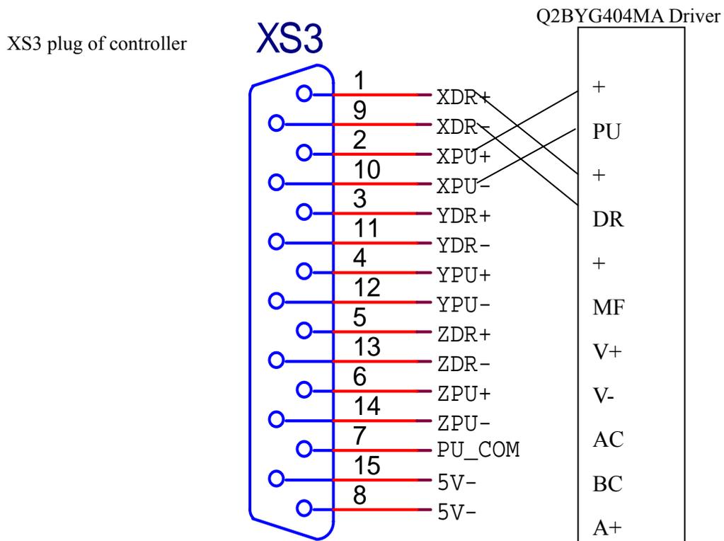
The following connecting diagram shows the connection of ADTECH Q2BYG404MA driver and 56BYGH630C stepping motor:
