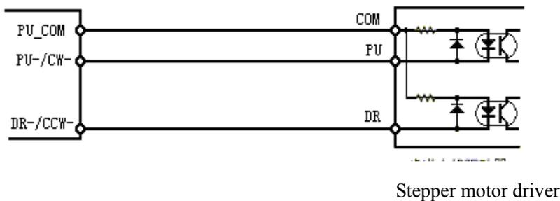
**Note: It is not applicable to the some stepper motor drivers whose pulse and direction cathodes are connected together.**
