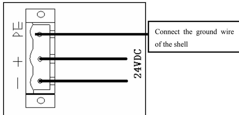
2) A magnetic loop should be used in the input line of NCS 24V power supply. As shown below:
