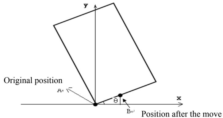
Press [X+] → [Y+], or [Y+] → [X+], then, press [ENTER] to confirm. The position of figure to be processed and the steel plate is shown as follows:
