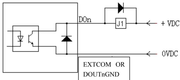
EXTCOM is connected to the negative end of internal power supply, and the output signal is connected to the relevant terminal.
