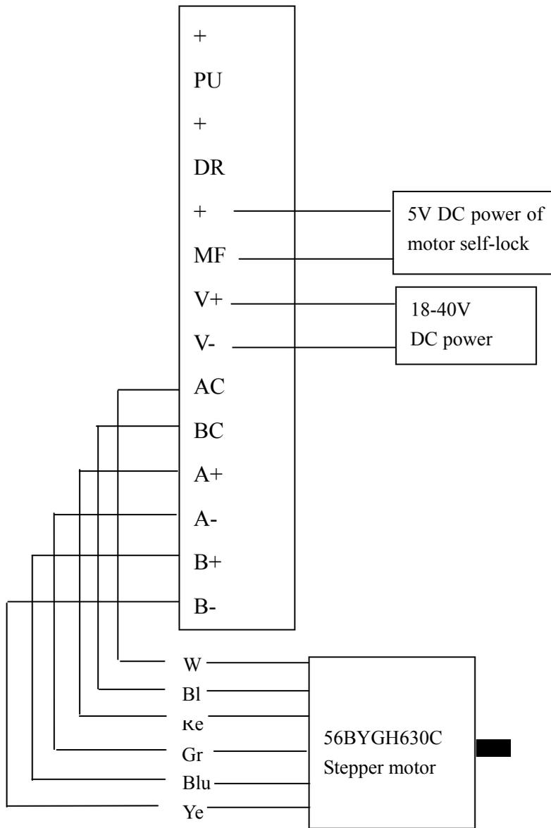
The following connecting diagram shows the connection of ADTECH Q2BYG404MA driver and 56BYGH630EJP stepping motor:
